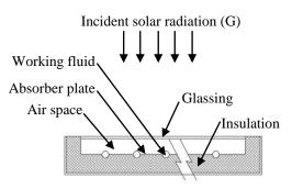
Fig. 1 Schematic diagram of flat-plate solar collector
