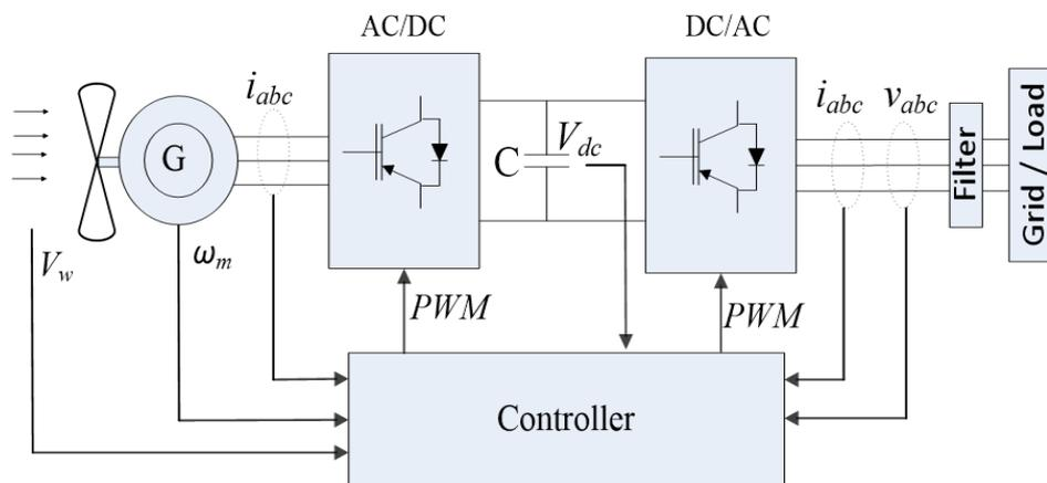
Fig. 1: Wind Energy Conversion System Diagram
