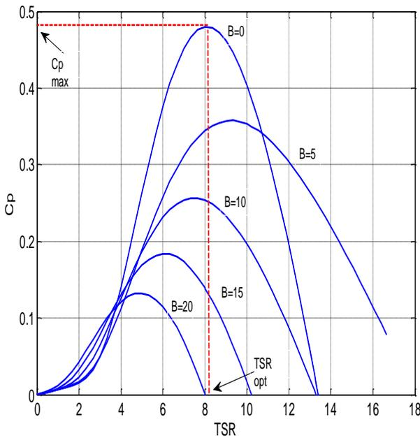
Fig. 2: Graph of power coefficient against TSR
