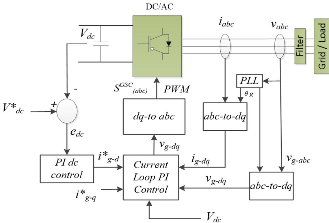
Fig. 5: The schematic diagram of the grid side PI control
