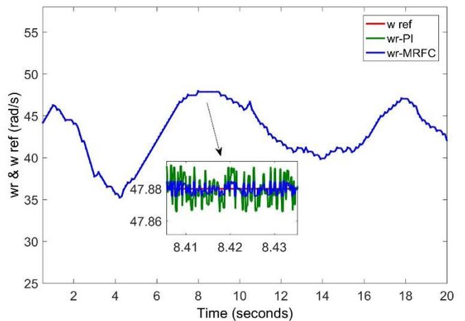
Fig.10: Tracking response of rotor with reference speeds for PI and MRFC
