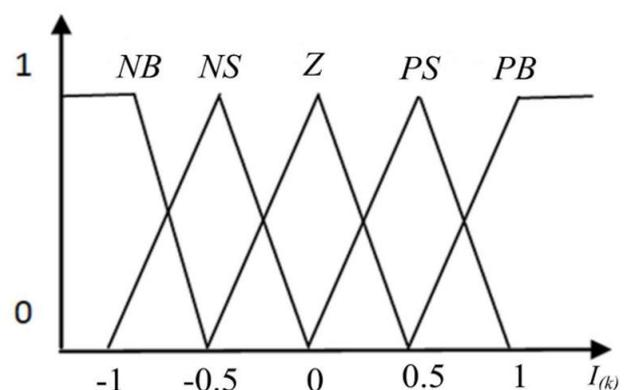
Fig. 8: Membership Function of output variables  $i_q$
