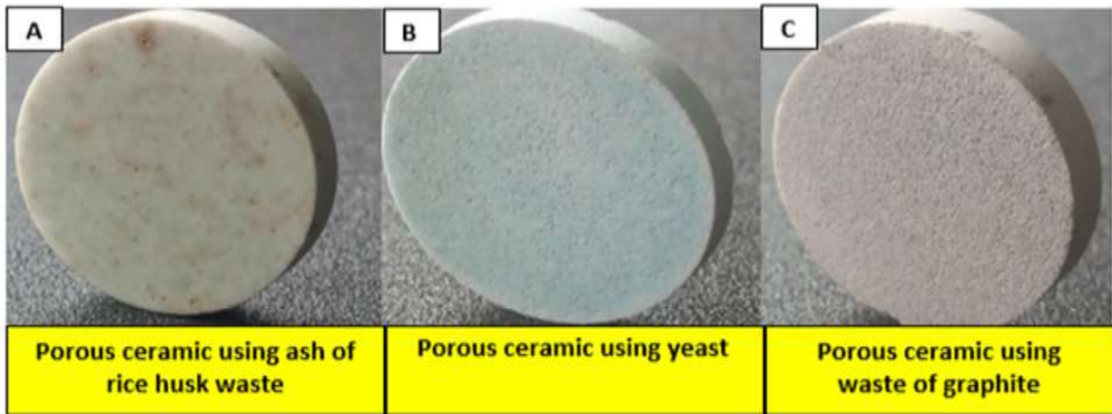
Figure 2. Porous ceramics specimens using three types of PFAs (A-ash of rice husk, B-yeast, and C-waste of graphite).
