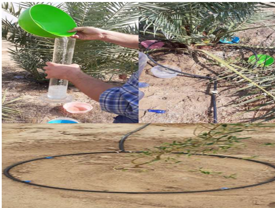
Figure 4: Measurement of the discharge from the drippers.
