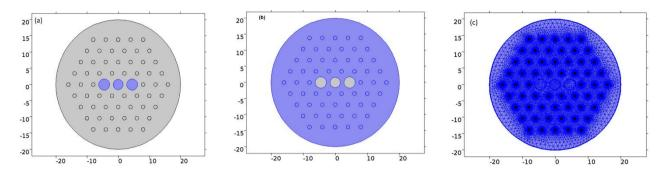
Fig. 1: Geometry structure of three-core photonic crystal fiber with three-ring hexagonal lattice: (a) insert core material; (b) insert the cladding material, (c) mesh free-triangular.
