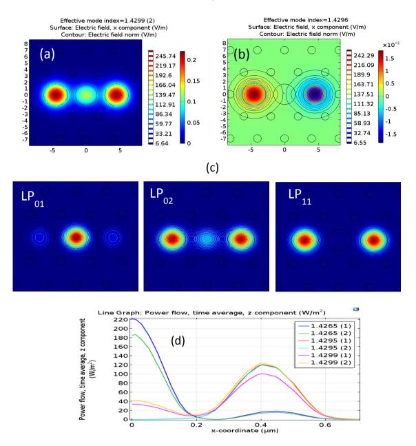
Fig. 4: Effective mode index and Surface: Electric field distributions of the x component for (a) Identical (b) Non-identical, three cores PCF coupler. (c) Power flow distributions of the six fundamental modes of the identical three-core PCF for core diameter of 3.2μm. (d) Power flow for the fundamental modes of the three cores at wavelength 1.55μm.
