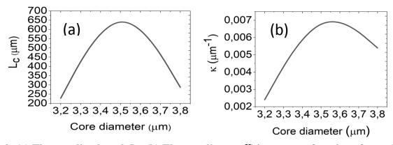
Fig. 2: (a) The coupling length  $L_C$  (b) The coupling coefficient  $\kappa$ , as a function of core diameter at wavelength 1550nm.
