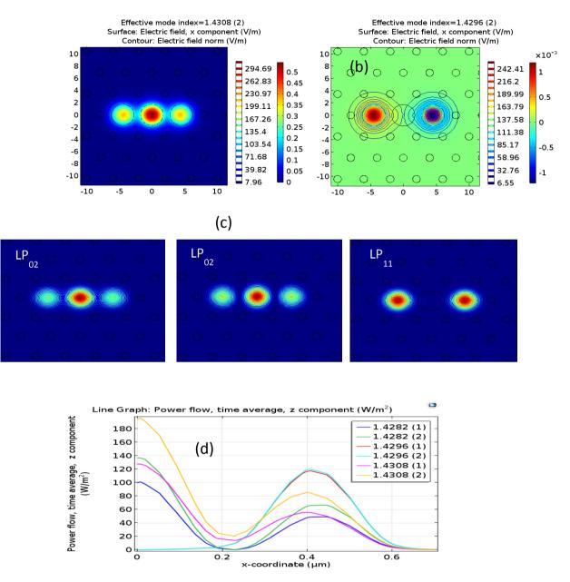
Fig. 3: Effective mode index and Surface Electric field distributions of the x component for (a) Identical and (b) Non-identical, three cores PCF. (c) Power flow distributions of the six fundamental modes of the identical three-core PCF for core diameter 3.5μm. (d) Power flow for the fundamental modes of the three cores at wavelength 1.55μm.
