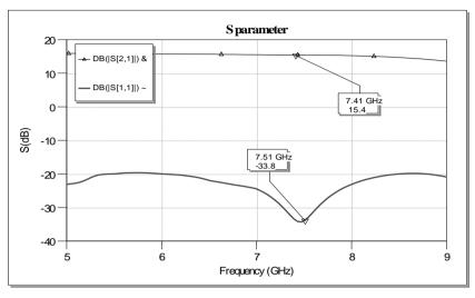
Fig. 12: The S-parameters indicate for FET circuit
