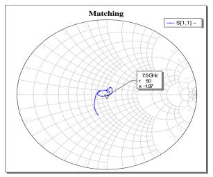
Fig. 11: Smith chart shows the matching at 7.5GHz for FET circuit
