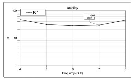
Fig. 14: The stability factor K>1 along operating frequency for FET circuit
