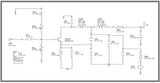
Fig. 9: The Lumped BJT circuit
