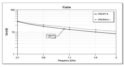
Fig. 6: The linear power gain for distributed BJT circuit
