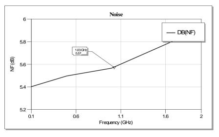
Fig. 8: Noise-Figure of BJT circuit
