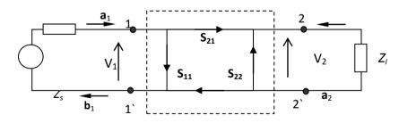
Fig. 1: The equivalent two port circuit
