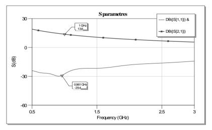
Fig. 5: S-parameters single BJT-stage lumped BJT circuit
