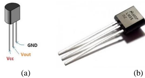
Figure 2: (a) Lm35 pinout (b) Lm35 sensor
