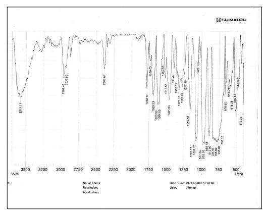
Fig. 2: IR chart for SILC-PMA ion pair .
