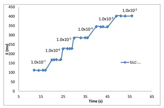
Fig. 6: Response time of SILC-PMA electrode.
