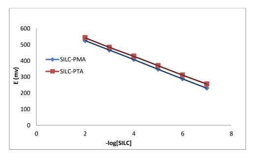
Fig. 3: Standard curve of SILC using new SILC-PTA and SILC-PMA electrodes.
