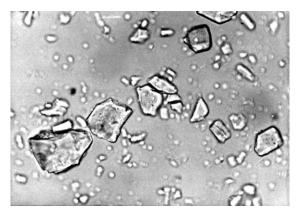
Figure (2): Microscopical examination of ZETA stone (Particles are regular, dense and prism–like)
