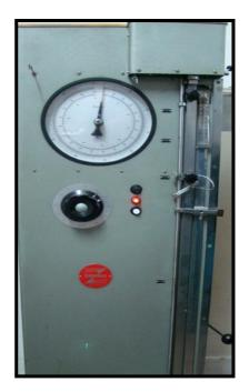
Figure (1): Tensile testing machine.
