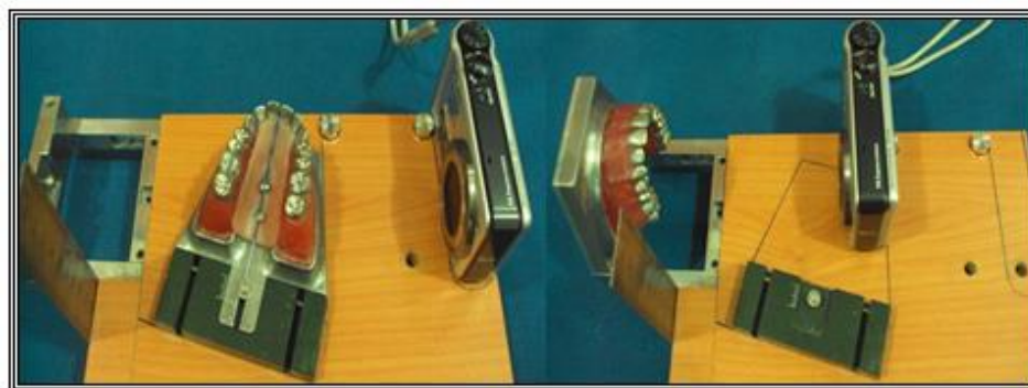
Figure (2): Wood table with two metallic bases to receive the typodont and digital camera
