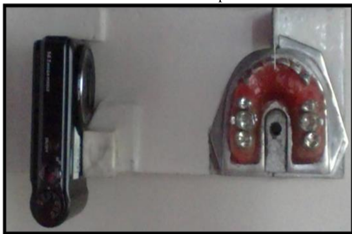
Figure (1): Wood table with the vertical and horizontal bars, custom made base for typodont and digital camera fixation.
