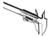
Figure (1): Sliding caliper with vernier scale
