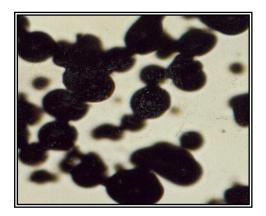
Figure (3): Vivacap alloy (×400). Small spherical particles
