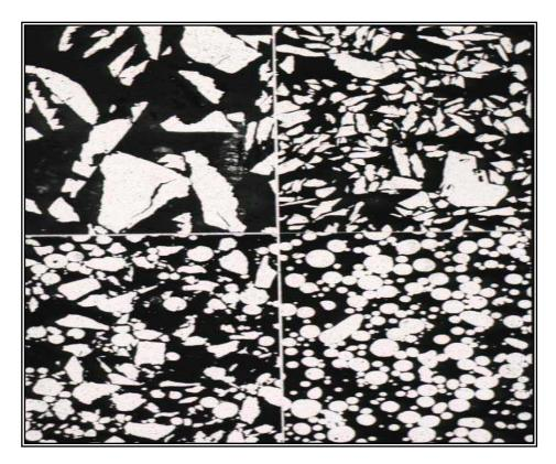
Figure (1): Different alloy particles shape<sup>(4)</sup>
