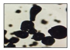
Figure (4): Aristaloy 21 alloy (×400). Mixed spherical and lathe–cut particles
