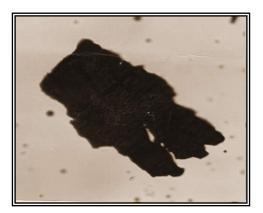
Figure (2): Al–Rafidain alloy (×400). Large irregular lathe–cut particles
