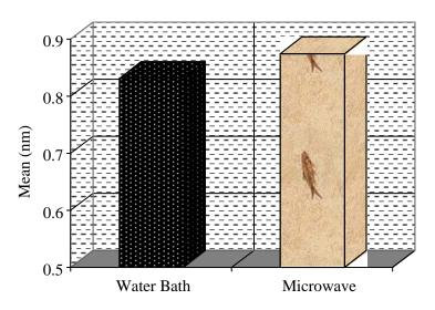
Figure (2): Optical density of colour of Major–base acrylic resin cured by two techniques
