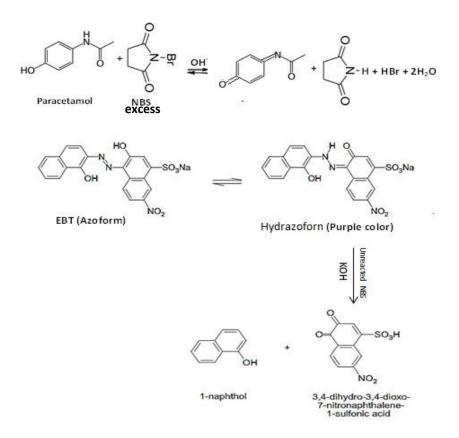
Scheme: Proposed mechanism for oxidation of EBT by NBS
