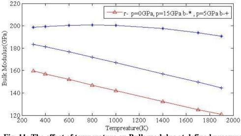
Fig. 11: The effect of temperature on Bulk modulus at defined pressure
