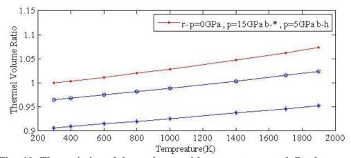
Fig. 10: The variation of thermal  $v_{p/V_0}$  with temperature at defined pressure
