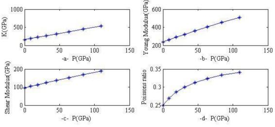
Fig. 2: Comparison of calculated elastic moduli with the resercher Results of (Upadhyay and Sharma , 2011)
