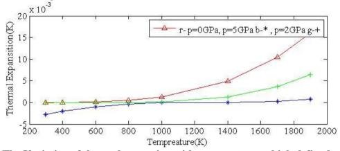
Fig. 9: The Variation of thermal expansion with temperature at high defined pressure
