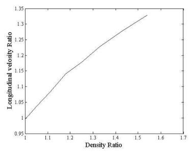
Fig. 6: Relation between longitudinal velocity ratio with Density ratio
