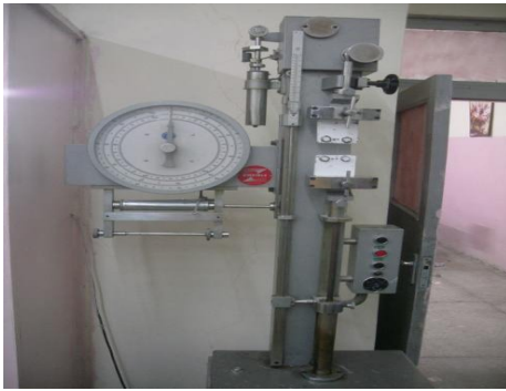
Figure (1): Device used in the tensile strength test.
