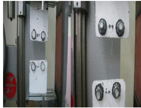
Figure (2): Before and after tensile test.
