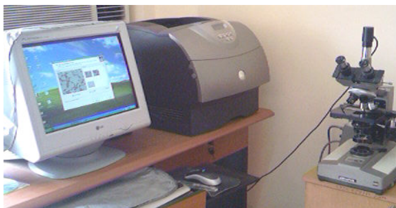
(Figure 1) Light microscope with camera connected to computer
