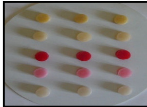
Figure: (4) Samples of different waxes used in flow, hardness and accuracy test.
