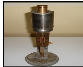
Figure: (2) Vicat apparatus After modification.
