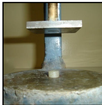
Figure: (6) Sample placed under the axial load of vicat apparatus.
