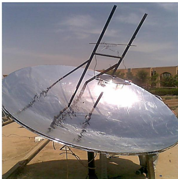
Fig. 1: Parabolic solar cooker used in the experiment.
