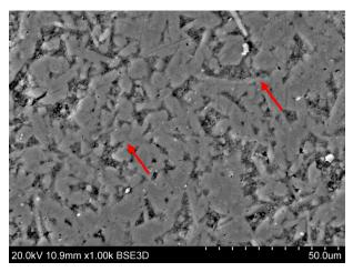
Figure (5): SEM of ZnO NPs specimens (0.5%) at 1000 x magnification.
