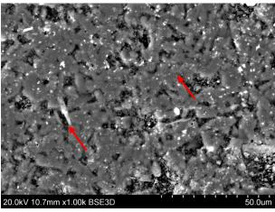
Figure (8): SEM of ZnO NPs specimens (2.0%) at 1000 x magnification.
