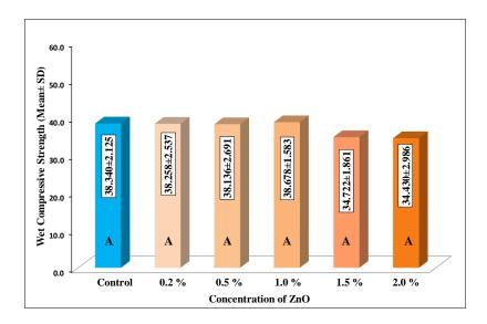
Figure (1): Mean ± SD Duncan's multiple range test of wet compressive strength of dental stone among different concentrations of ZnO NPs.
