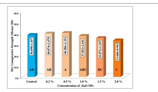
Figure (2): Mean ± SD Duncan's multiple range test of dry compressive strength of dental stone among different concentration of ZnO NPs.
