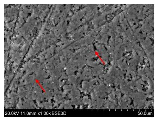
Figure (4): SEM of ZnO NPs specimens (0.2%) at 1000 x magnification.
