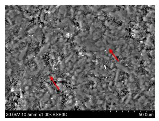
Figure (7): SEM of ZnO NPs specimens (1.5 %) at 1000 x magnification.
