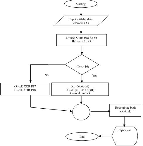
Figure 3: The Flow Chart of Blowfish Algorithm
