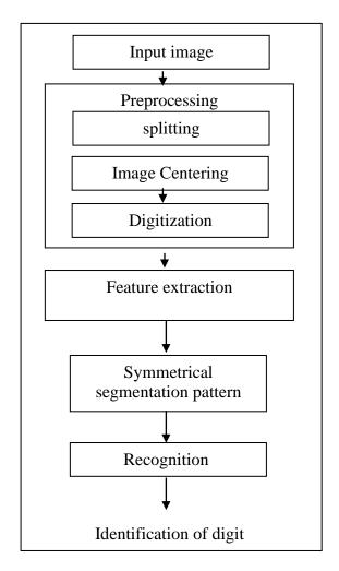
Figure -2 Block diagram of the proposed system
