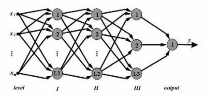
Figure (1) Architecture of the feedforward neural network. **3. Advantages of Using Artificial Neural Networks:**
