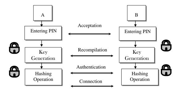
Figure 4: The Authentication & Hashing operation
