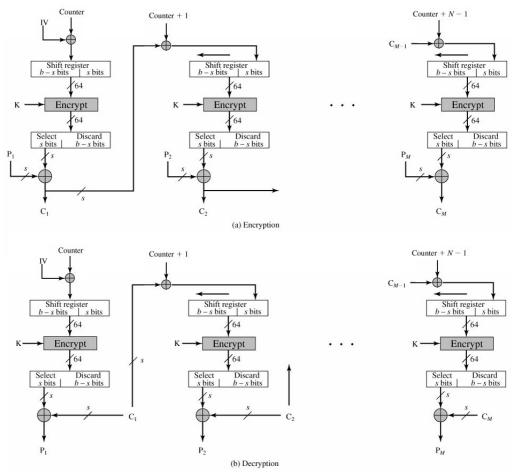
Fig.3: s-bit Counter Cipher Feedback (CCFB) Mode
