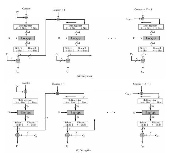
Fig.4: s-bit Counter Output Feedback (COFB) Mode
