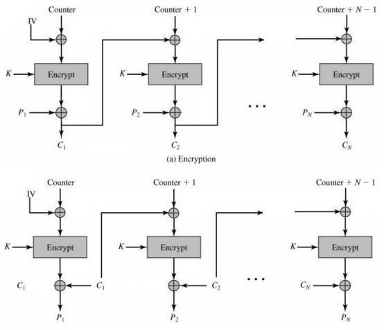
Fig.2: Counter Cipher Block Chaining (CCBC) Mode
