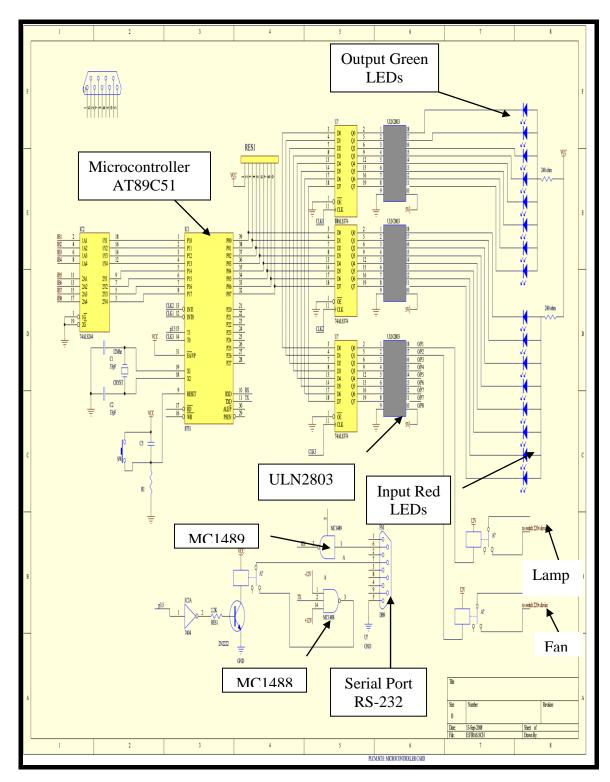
Fig.(2) The Schematic Diagram of Board 1
