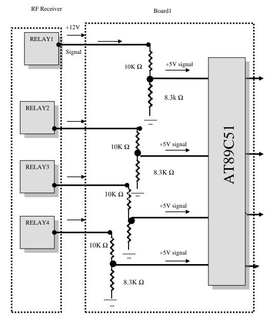
Fig.(4) Interface Between RF Receiver and AT89C51 in Board 1
