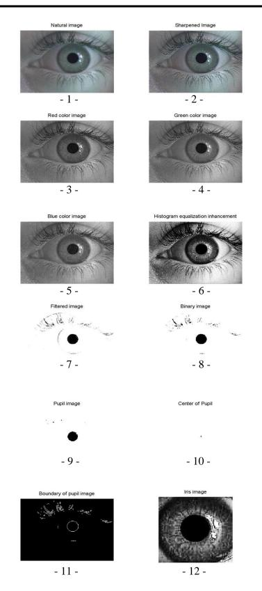
Figure (6): Steps of analysis from picture acquisition of eye until iris localization and extraction
