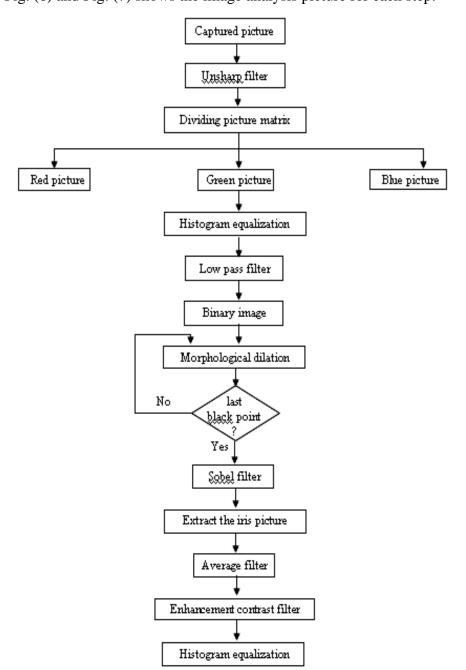
Figure (5): The block diagram of the steps adopted in the analysis of the eye image
