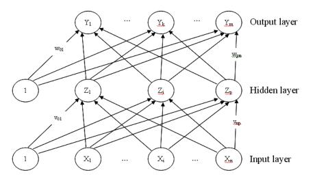
Figure (8): Backpropagation neural network with one hidden layer.
