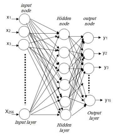
Figure (4): structure for Fuzzy BackPropagation Network (FBPN)
