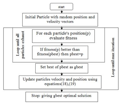
Figure (3) : Flow chart for Particle Swarm Optimization (PSO)
