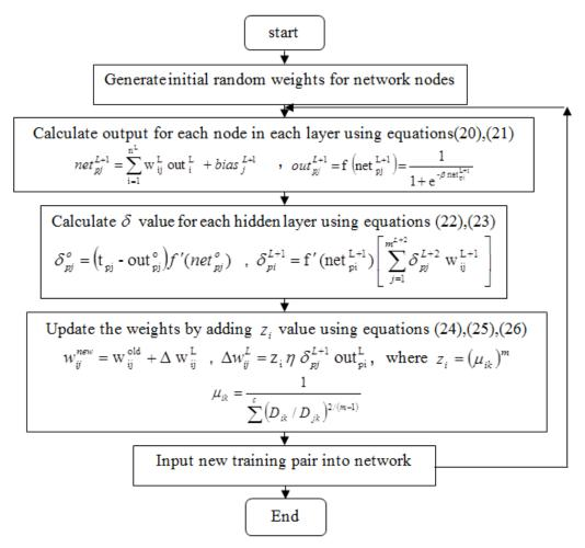
Figure (5) : Flowchart for Fuzzy BackPropagation Network (FBPN) Algorithm
