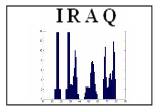
Figure (3): Using vertical histogram to truncate characters
