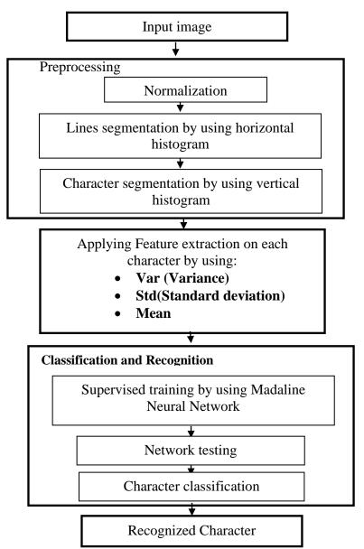
Figure (1): The structure of the character recognition system
