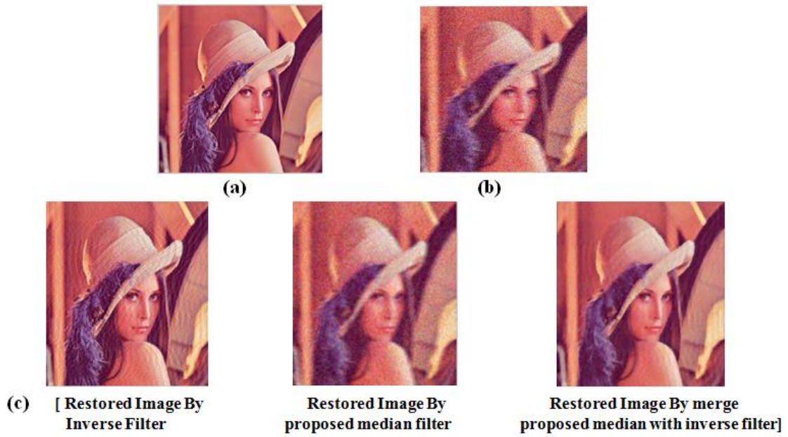
Fig.(3): (a) Original Image, (b) Image with Noise Gaussian & Blur Motion and (c) Reconstructed image of Lena.
