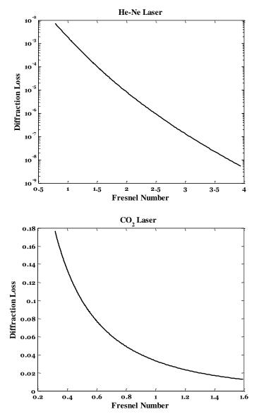
Figure(4): Diffraction Losses versus Fresnel Number for He-Ne & CO<sub>2</sub> lasers
