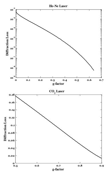
Figure(5): Diffraction Losses as a function of g-factor for He-Ne and CO<sub>2</sub> lasers
