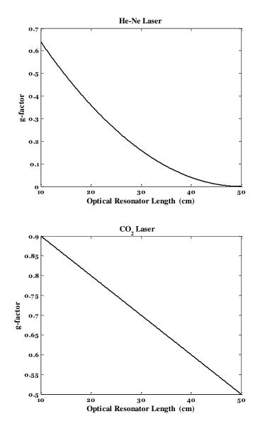
Figure(1): g-factor as a function of optical resonator length for He-Ne & CO<sub>2</sub> lasers
