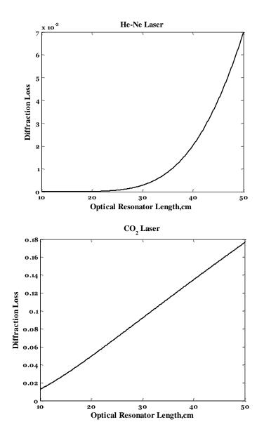
Figure(3): Diffraction Losses as a function of optical resonator length for He-Ne & CO<sub>2</sub> lasers
