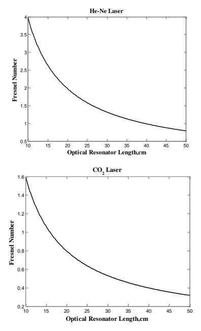
Figure(2): Fresnel Number as a function of optical resonator length for He-Ne & CO<sub>2</sub> lasers
