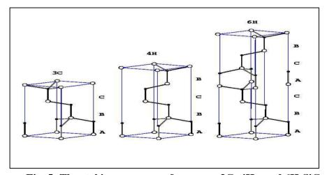
Fig. 5: The staking sequence of common 3C-,4H-, and 6H-SiC
