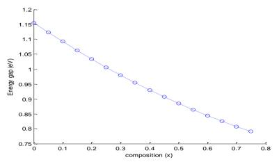
Fig. 7: Energy gap for Si<sub>1-x</sub>Ge<sub>x</sub> at different composition at room temperature
