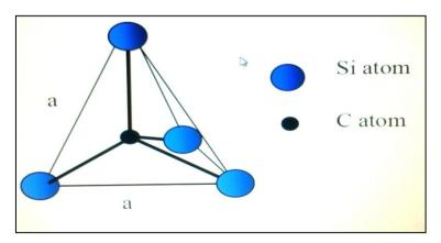
Fig. 3: The tetragonal bonding of a carbon atom with the four nearessilicon(Lee, 2002).
