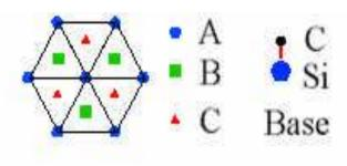
Fig. 4: The staking sequence of silicon carbide
