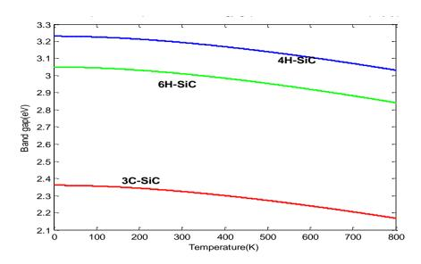
Fig. 2: Temperature dependence of energy gap for 3C-, 4H-, and 6H-SiC polytypes at atmospheric pressure
