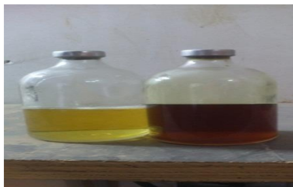
Figure,1: Changing in color after the reduction of \text{Ag}^+ to SNPs by Salvia officinalis 's plant leaves extract at (1-8hrs).
