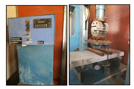
Plate 3. Photo of Concrete Flexural Machine used in this test
