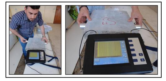
Plate 7. Ultrasonic Pulse Velocity (UPV) Test
