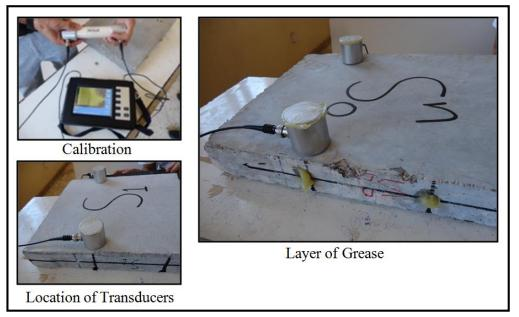
Plate 4. Details of UPV Test
