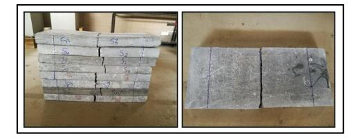
Plate 6. Final Failure for All Specimens
