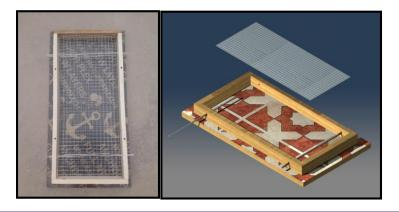
Figure 1. The Mould That Used in This Test
