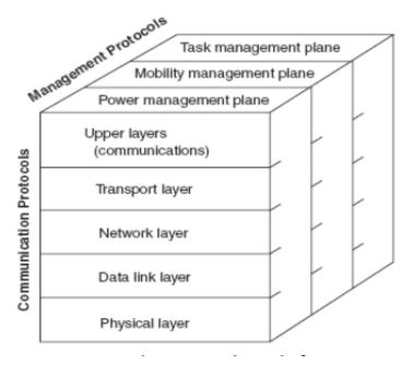
Figure 3. Representation of Generic Protocol Stack for wireless sensor Networks
