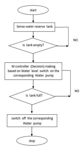
**Figure 8:-flowchart for Intelligent tank**
