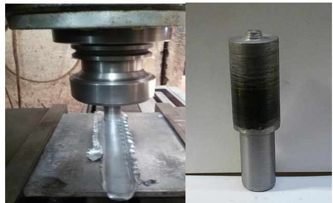
Figure 1: Sample after frictions stir processing
