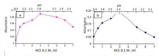
Figure 2: Effect of pH on the absorbance of  $25\mu$ g/ml Ibuprofen (a) and  $8\mu$ g/ml Nystatin (b) ion pair complexes with 2.5 ml of  $3\times 10^{-3}$  M C2R dye.
