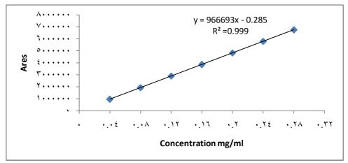
Figure 3. Calibration curve for tadalafil.
