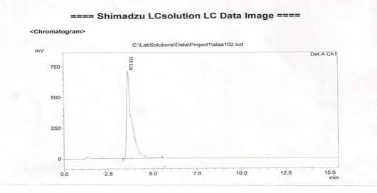
Figure 2. Typical chromatogram (tadafil 0.16mg/ml)
