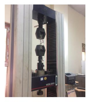
Fig. 3 The tensile test machine used.
