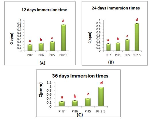
Figure(1):mean,±standerd deviation and Multiple Comparisons of Cr release s in solution dependent on the pH after various immersion times, (A:12 days immersion time, B: 24days immersion time,C: 36 days immersiontime).
