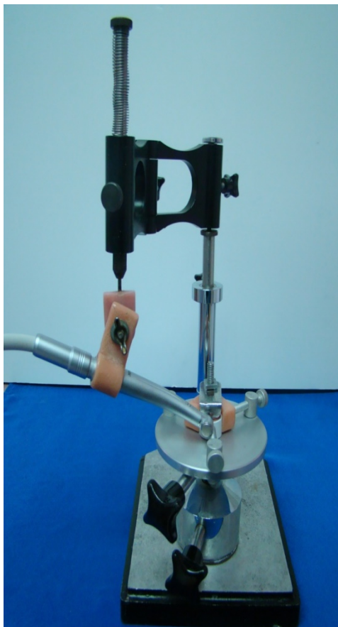
Figure(1): Sample with stationary hand piece secured in a clamp attached to a surveyor.
