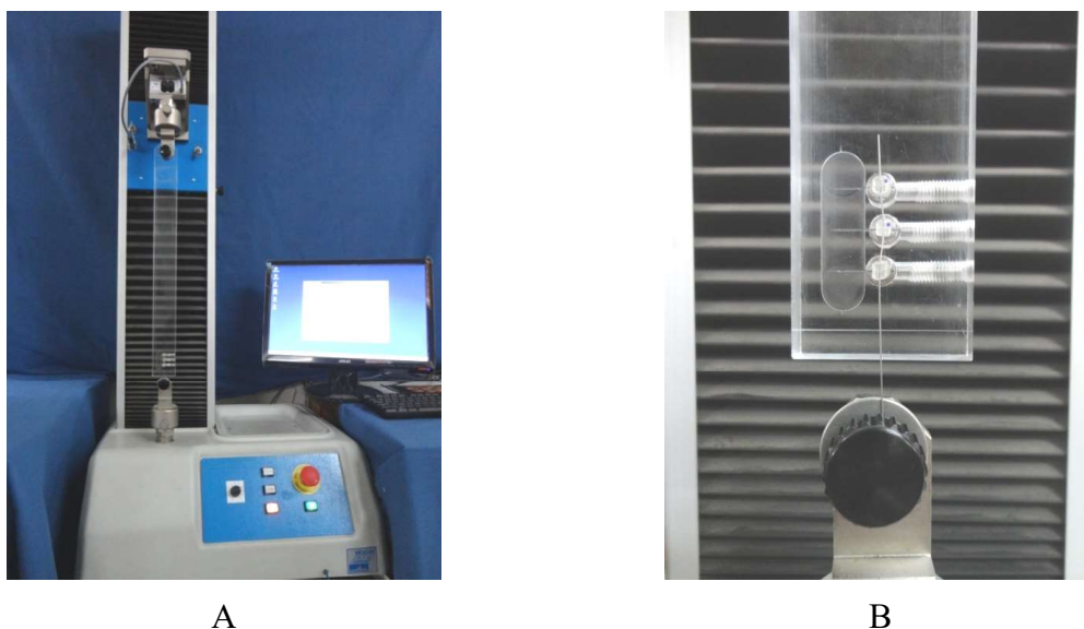
Figure (1): Setup of Experimental Model on the Tensile Testing Machine
