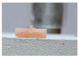
Figure (1): Drop of deionized water on flexible denture base sample
