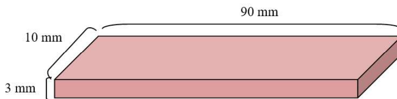
Figure (2): Tensile testing sample dimensions
