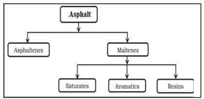
Fig. 1: (SARA) Parts separated from asphaltMaterials
