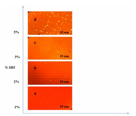
Fig. 12: Image of SBS PMA sample with 400 magnifications
