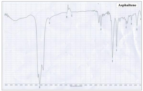
Fig. 5: IR spectrum for asphaltene
