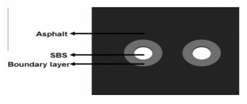
Fig. 3: Modification mechanism of SBS modified asphalt
