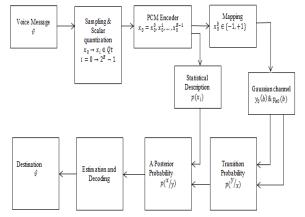
Figure 1: Block diagram of proposed PCM communication system
