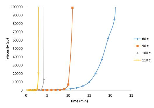
Figure 3. Viscosity versus time at different temperatures and 21.00phr.
