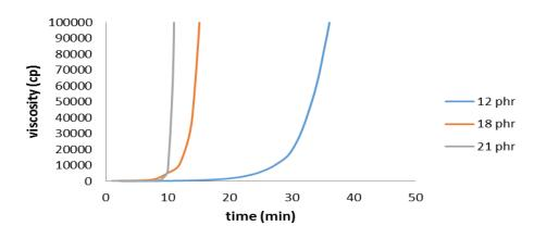
Figure 5. Viscosity vs gel time with differ cure composite at 90 °C.
